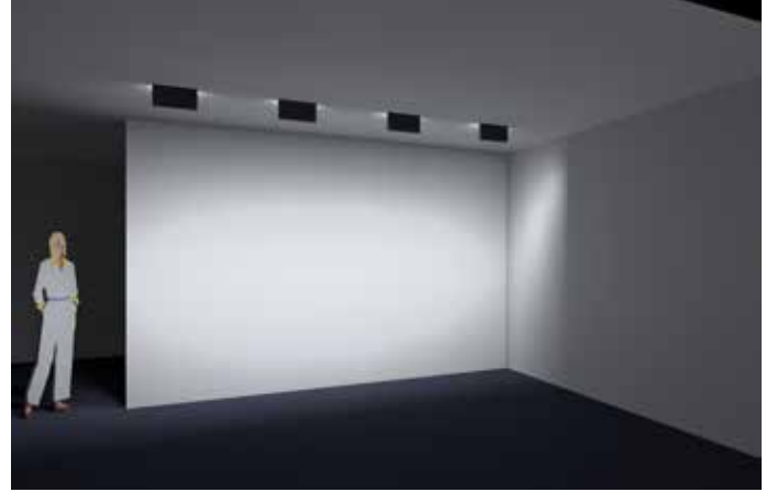
Simulation of a classical wall washer light solution. Uneven wall illumination at high glare.
